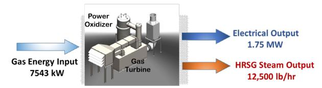
The diagram below shows the calculated<sup>\*</sup> net CO<sub>2</sub> emissions benefit to Pacific Ethanol of avoiding grid electricity purchases, using the cogeneration facility's steam to offset pipeline gas purchases and destroying the process by-product VOCs in the Ener-Core oxidizer. The VOC destruction avoids 2 MMBtu/hr or almost 17,000 MMBtu of gas purchases each year.
