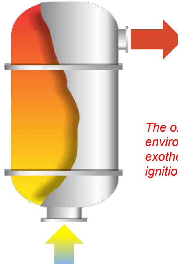
Ambient air + waste gases are introduced to vessel
